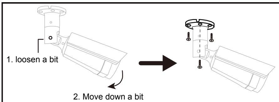
Step 2: Adjust the viewing angle of the camera as indicated below.
